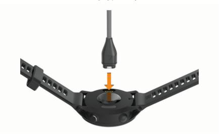
2 Plug the large end of the USB cable into a USB charging port. The watch displays the current battery charge level.
